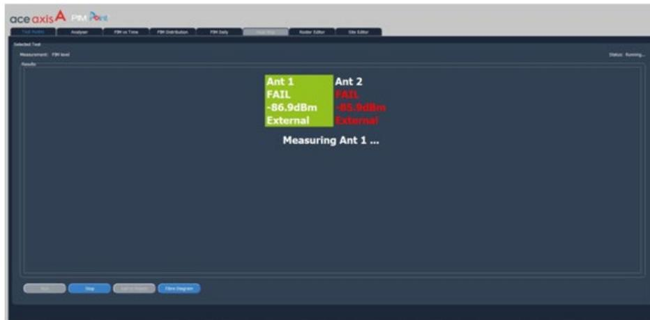
**Monitoring mode** – the equipment is left at the cell site to monitor the rise and fall of PIM level with the actual traffic at the cell site. This allows the identification of sites where PIM is causing a problem under normal operating conditions. An event log is created to allow the Operator to quickly and precisely see the time, duration and amplitude of the PIM and make a quick decision to invest money & resources to fix (or leave) the PIM problem.
