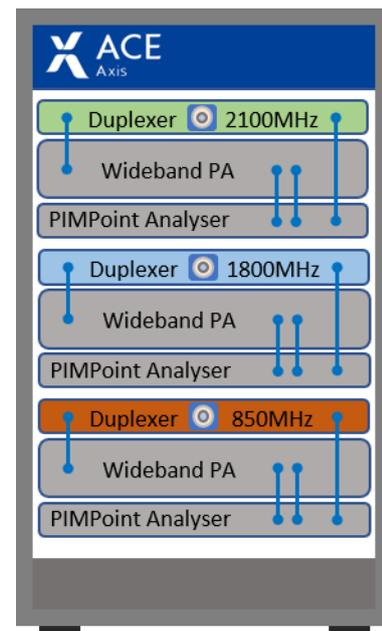
Multi-band test station configured for 850MHz, 1800MHz and 2100MHz bands
