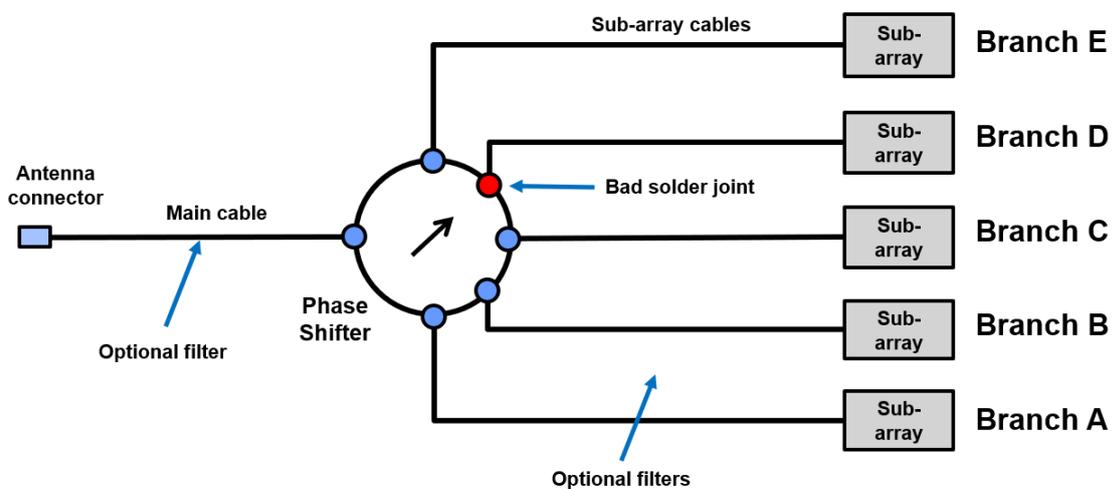
Location is by branch (A to E) and by component type from left to right (Antenna connector, phase shifter or radiating element or sub-array) giving a totally new dimension to PIM measurement capability. Sometimes antennas may also include filters or diplexers or other functions at the locations indicated and in many cases faults at these components may also be identified.
